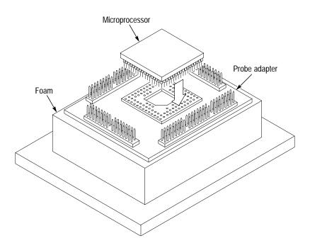
Figure 1–3: Placing a microprocessor into the conventional probe adapter
