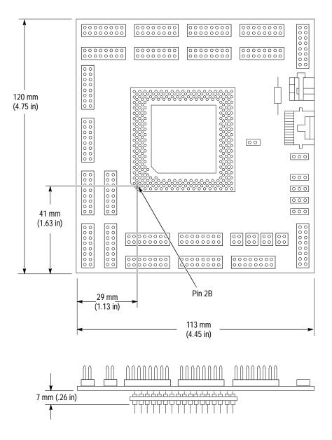
Figure 3-2: Dimensions of the conventional probe adapter
