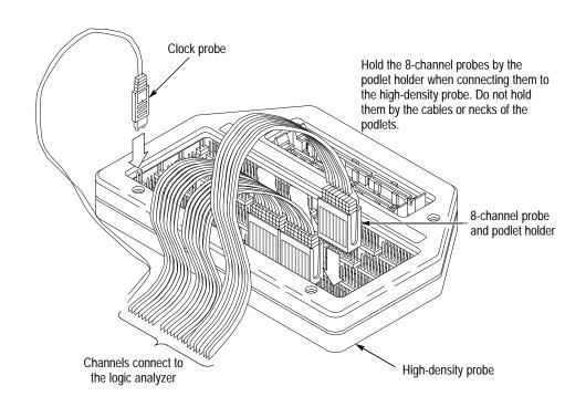
Match the ground pins on the probes to the corresponding pins on the probe adapter.
