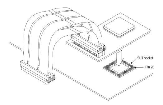
Figure 1–7: Placing the low-profile probe adapter onto the SUT
