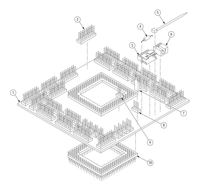
Figure 1: P54/P55 conventional probe adapter exploded view
