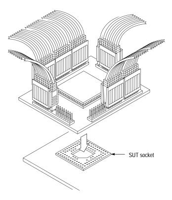
Figure 1–5: Placing the conventional probe adapter onto the SUT
