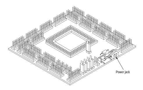
Figure 1–10: Power jack location on the conventional probe adapter
