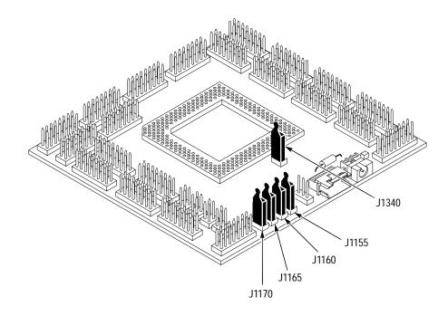
Figure 1–1: Jumper locations on the conventional probe adapter
