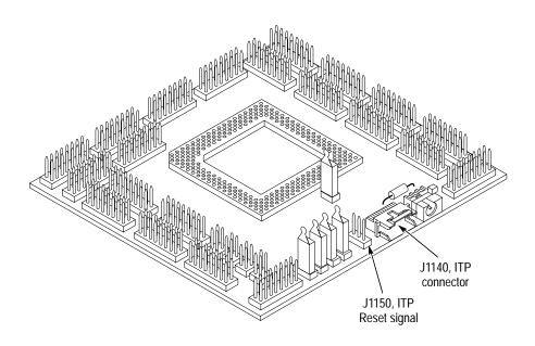
Figure 3-5: Location of J1140 and J1150 on the conventional probe adapter
