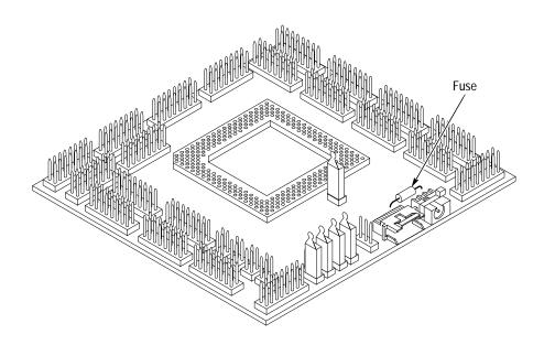
Figure 4–1: Location of the fuse on the conventional probe adapter
