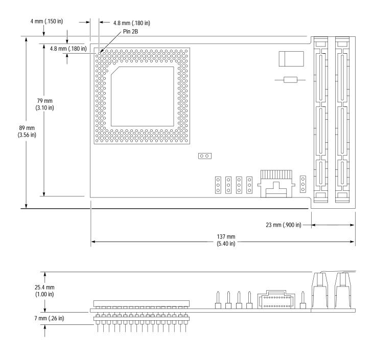
Figure 3–1: Dimensions of the low-profile probe adapter
