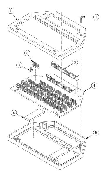
Figure 3: 192-Channel High-Density probe exploded view
