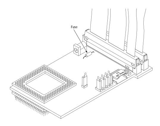
Figure 4-2: Location of the fuse on the low-profile probe adapter
