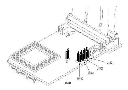
Figure 1–2: Jumper locations on the low-profile probe adapter
