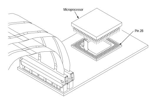
Figure 1–6: Placing a microprocessor into the low-profile probe adapter
