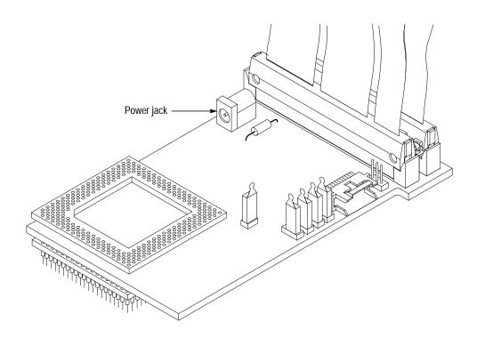
Figure 1-11: Power jack location on the low-profile probe adapter
