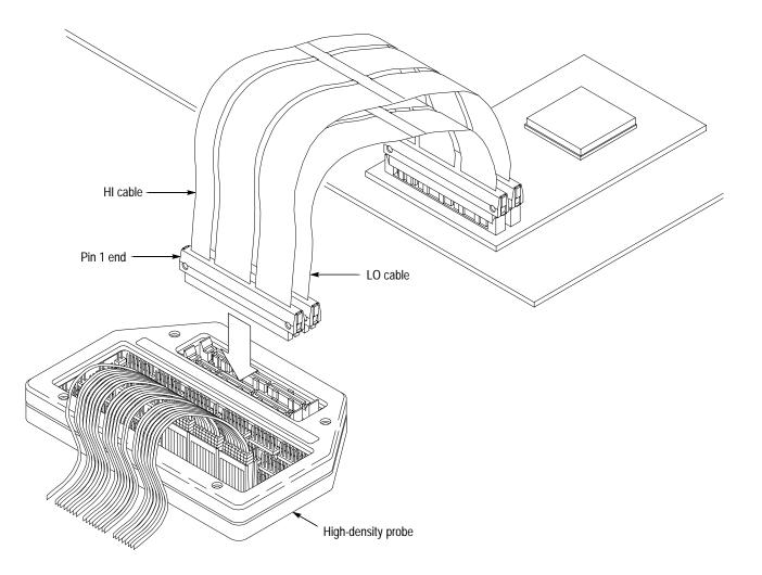
Figure 1–9: Connecting LO and HI cables to a high-density probe
