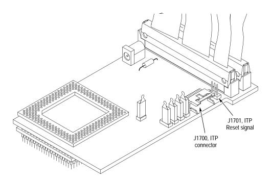
Figure 3-6: Location of J1700 and J1701 on the low-profile probe adapter
