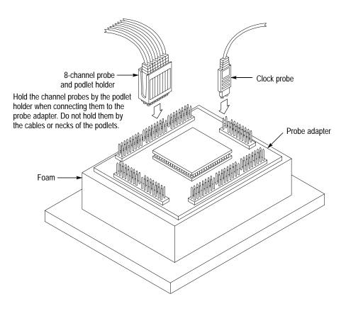
Figure 1-4: Connecting probes to the conventional probe adapter
